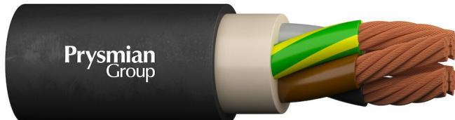
OZOFLEX™ rubber cables are suitable for dry as well as humid or moist environments, in- and outdoors. They are extreme flexible, hardwearing and oil-resistant. OZOFLEX™ cables are also appropriate for fixed installations up to 1000 V AC in conduit or appliances, as well as for connection of hoisting motors.
